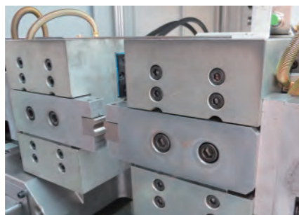
高精度自定心同步夹持系统 High accuracy self centering synchronous clamping system
