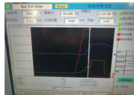
焊接曲线 Welding curve
